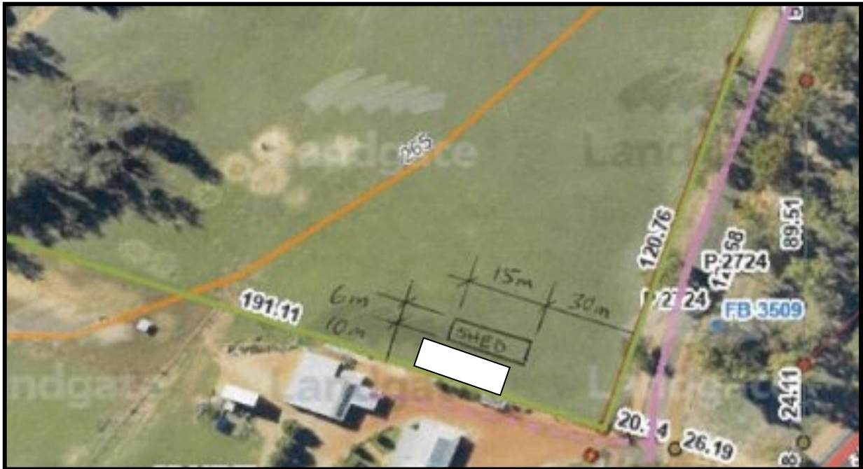
Aerial – Not Accurate or to Scale. Partial site plan showing outbuilding in south east portion of the lot
